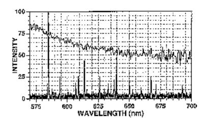
Comparison of the spectrum of SL from a 3 Torr neon bubble and the spectrum of gas discharge through a 75 Torr neon atmosphere. Note that the dramatic peaks which give neon its characteristic orange-red colour are absent for SL.
