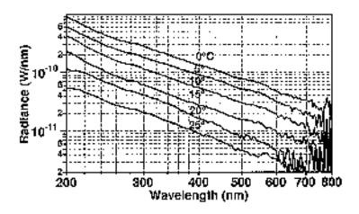
Corrected spectra for a 150 mm bubble of helium in water at various temperatures.
