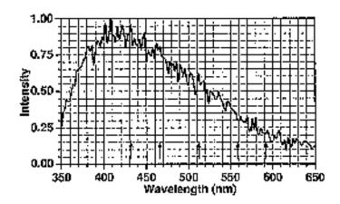
Spectrum of xenon in dodecane. Obtained at a resolution of 1 nm, this spectrum shows no evidence of the Swan lines which are emitted by excited carbon molecules. Swan lines have been observed in experiments designed to measure transient SL.
