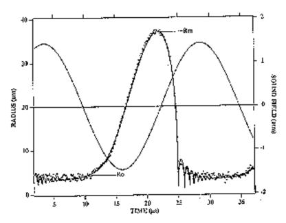
Radius of a 3 mm xenon bubble as a function of time over one acoustic cycle. When the acoustic pressure is negative the bubble expands. This is followed by collapse and ringing before the bubble sits dead in the water waiting for the next cycle. Calibrating the data by the Rayleigh-Plesset equation (solid line) the ambient radius is 4.3 microns and the acoustic overpressure is 1.45 atmospheres.
