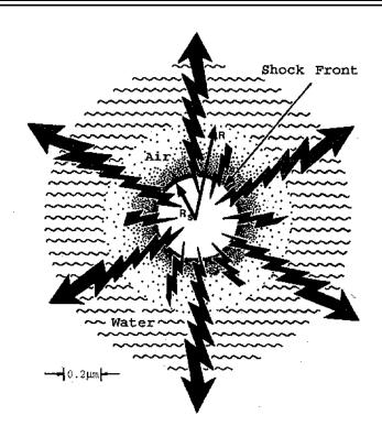
Sketch of an imploding shock wave model of SL. The shock is launched by the supersonic motion of the bubble wall. The radius of the gas water interface is R and the radius of the shock is  $R_s$ . The shock first implodes to a focus and then explodes. This figure depicts the state reached about 100 ps after focussing.
