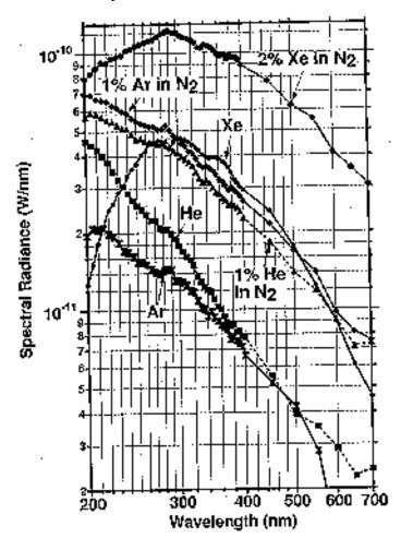
Spectrum of SL for various gas mixtures dissolved in water at T = 24 Celsius. (All for  $R_{ambient} = 150$  mm.) Note that although helium is dimmer than xenon it has higher spectral density in the ultraviolet.
