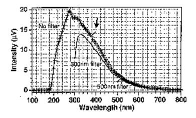
Raw data showing the uncalibrated spectrum of light emitted by a sonoluminescing bubble of helium in water. Note that spectral response turns on at about 185 nm (6.5 eV).
