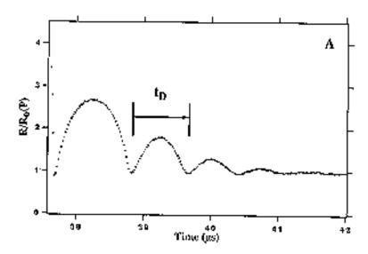
Detail of the bubble motion R(t) near the minimum radius  $R_{min}$ , taken with continuous laser illumination. The observation that  $R_{min}/R_{ambient} < 1/8$  indicates that the van der Waals hard core of the gas plays a role in limiting collapse of the bubble. The breathing period is  $t_D$ , and the time to go from the ambient radius to the collapse radius is  $t_E$ .
