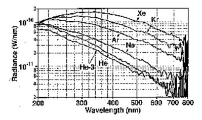
Room temperature spectra of various noble gasses in water.
