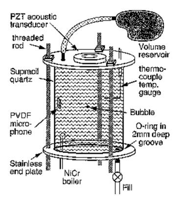
Sketch of a cylindrical resonator for obtaining sonoluminescence from a sealed system. This is important for controlling the composition and the partial pressure of the gas content in the resonator. The NiCr (toaster) wire is used to seed a bubble by boiling the liquid locally. The vaporous cavity fills with whatever gas is dissolved in the liquid, and is at the same time yanked to the velocity node of the sound field where it emits light at a sufficiently high acoustic drive.
