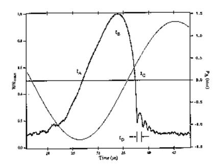
The radius R(t) scaled to the maximum radius  $R_{max}$  during one acoustic cycle. The experimental data comes from an air bubble in water. Comparison with the Rayleigh-Plesset equation of bubble dynamics indicates that for these data  $R_{ambient} = 4$  microns, and the amplitude of the acoustic overpressure is 1.35 atmospheres.
