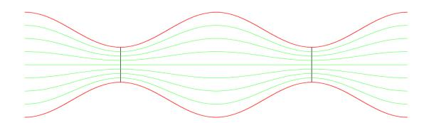
A second Laval nozzle is needed to bring the fluid flow back to subsonic speed [breakdown shock].
