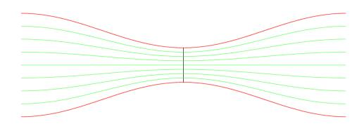
A Laval nozzle can be used to induce supersonic fluid flow. The acoustic horizon forms at the narrowest point of the nozzle.
