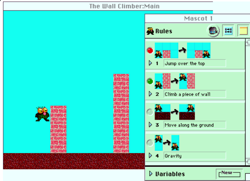
Figure 4: A Cocoa wall-climber (The Wall Climber: Main window) is following the rules (Mascot 1 window) that have been demonstrated for it. Each rule is shown with the graphical precondition on the left of the arrow and the graphical postcondition on the right of the arrow. The wall climber has just finished following rule 2, which places it in a position suitable for following rule 1 next.
