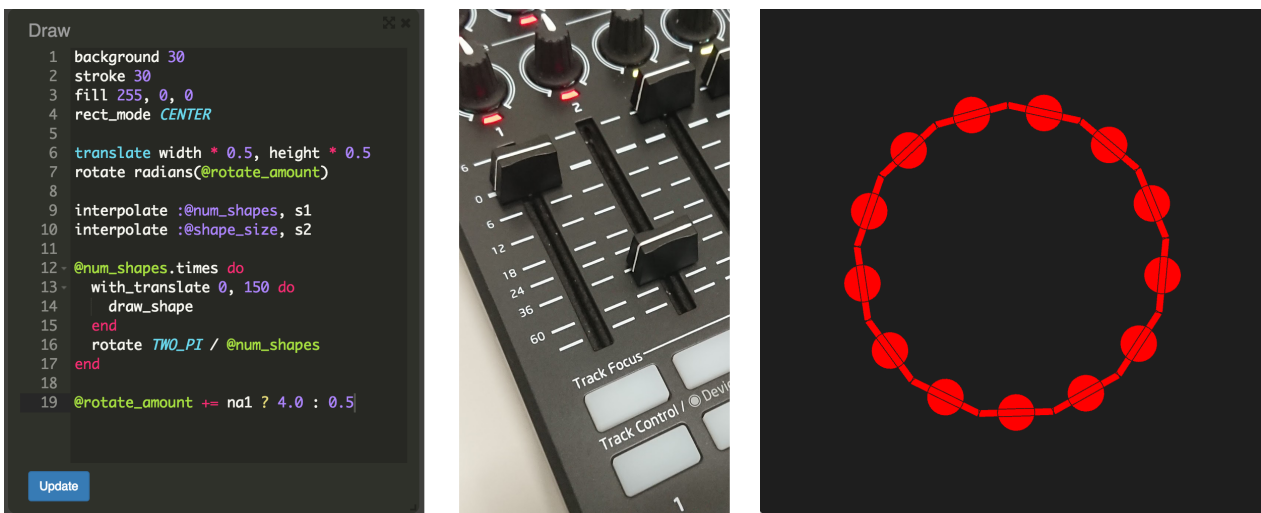
Figure 5: State manipulation by MIDI controller in Visor. Draw loop editor (left), MIDI controller (center) and the rendered output (right). Note how sliders have been assigned to the state variables using the interpolate method in combination with the s1 and s2 (lines 9 & 10) methods and how moving the sliders has affected the rendered output.
