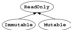
Figure 1: The hierarchy of immutability parameters, which have special meaning when used as the first type argument, as in List<Mutable, T> . (See also Fig. 6 in Sec. 2.4.)
