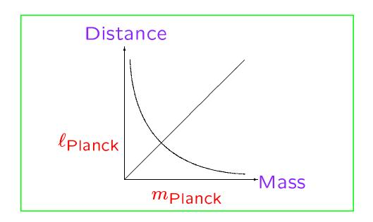
The Planck scale is the crossing point of Compton wavelength and Schwarzschild radius as a function of mass.
